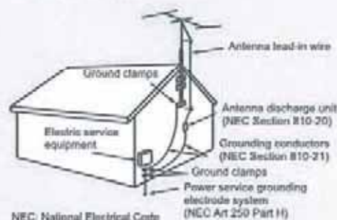
Antenna Grounding According to the National Electrical Code, ANSI/NFPA 70
